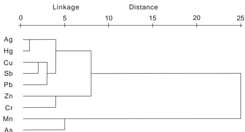
Fig. 3. Hierarchical dendrogram for 9 elements obtained by War's hierarchical clustering method (the distances reflect the degree of correlation between different elements).
